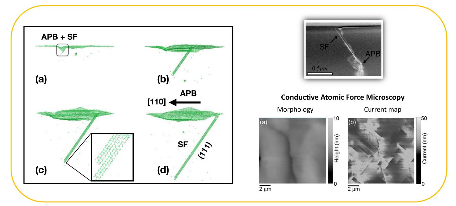
In our work [1] we focused on the atomic mechanisms ruling the extended defect kinetics in cubic SiC (3C-SiC), manifesting both stacking and anti-phase instabilities.
